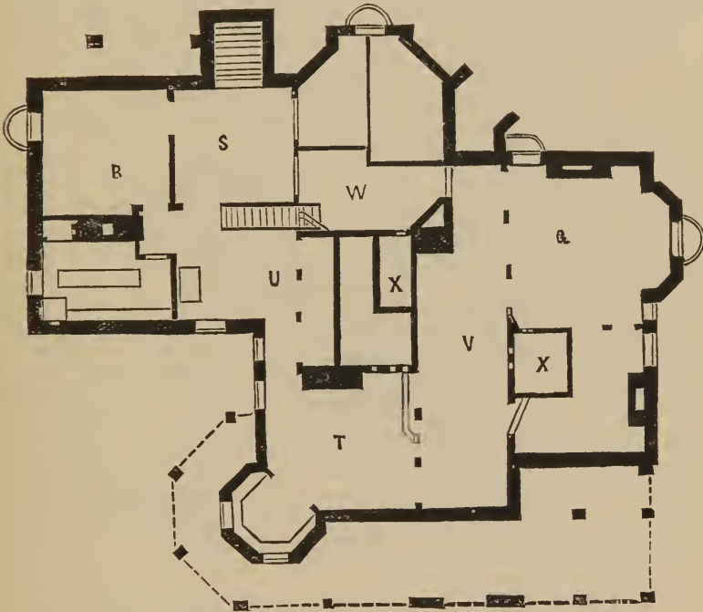
FIGURE 6.—CELLAR PLAN OF SUBURBAN HOUSE.—(See page 64.) Q.—Cellar. | S.—Stairs to Area. R.—Vegetable Store-Room. | W.—Entrance to Coal Vault. X.—Heating Coils.
